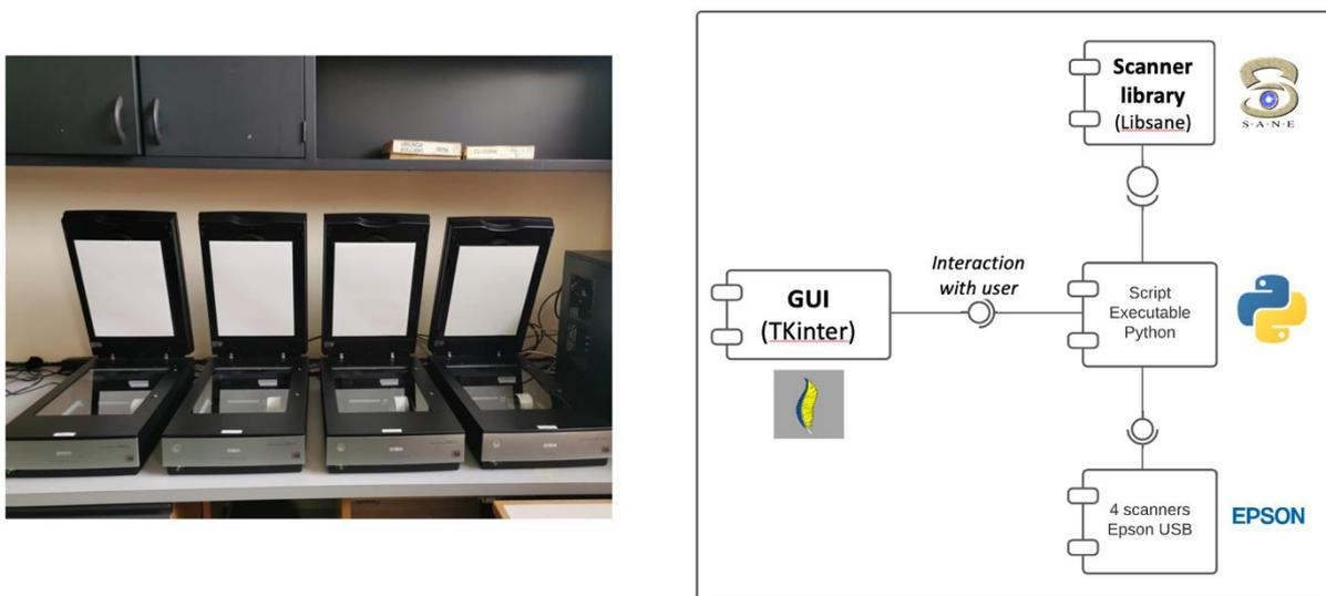
**Figure 11.** Mass-scanning infrastructure of the RMCA. Four flatbed photo scanners (photo on the left) digitise the historical aerial photographs in parallel, using the SANE library and a Python script (scheme on the right).
