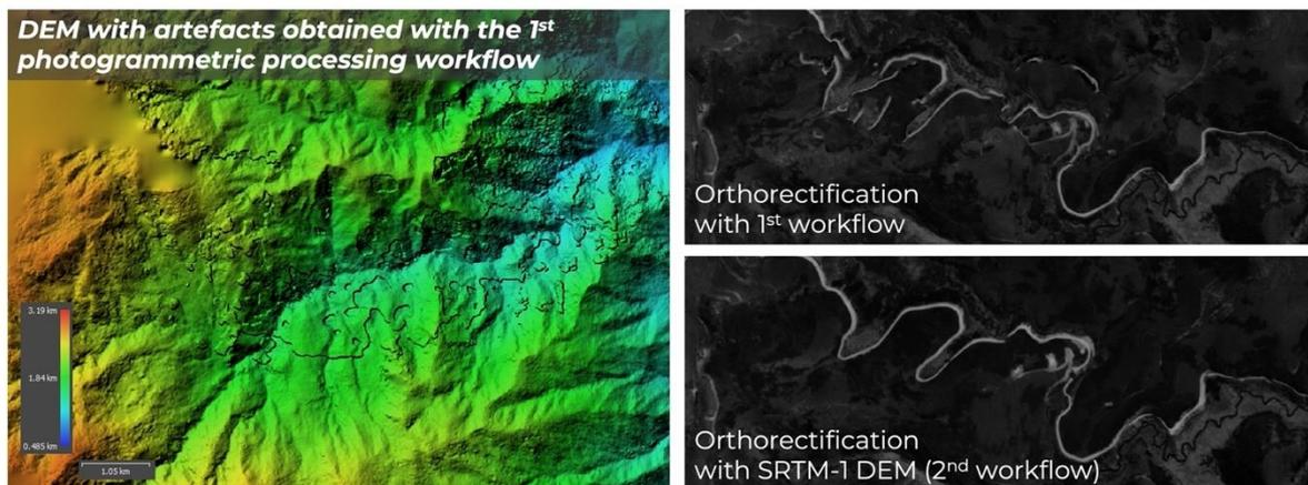
**Figure 15.** Comparison of the two photogrammetric workflows for low quality datasets, in mountainous environment. The left frame shows artefacts in a DEM derived from the aerial photographs, when image overlapping is insufficient. The frames on the right show how bad topographic reconstruction can lead to errors in the orthomosaic (top-right image), while an external DEM can solve most of these errors when it is used for orthorectification.
